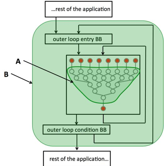
**Figure 2: State of the art identification algorithm traditionally focus on dataflow computation only (subgraph A). In this paper, instead, the control flow graph (CFG) of the application is also analysed, in search for static control parts (SCoPs) — subgraphs of the CFG where the flow of control is known *statically*. The whole SCoP region (subgraph B) is hence identified and selected as accelerator.**
