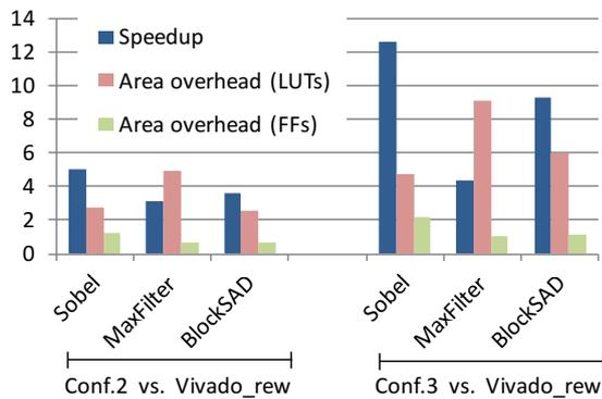
**Figure 7: Comparison of multi-datapath and optimised Vivado implementations.**
