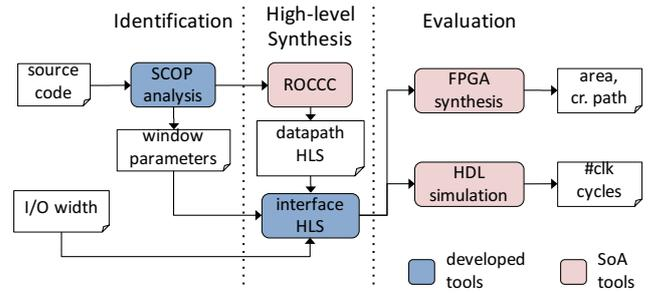
**Figure 1: Block scheme of our framework. Code analysis retrieves the parameters of SCoP kernels, which are employed, along with input/output constraints, to guide the automated design of highly efficient hardware accelerators.**
