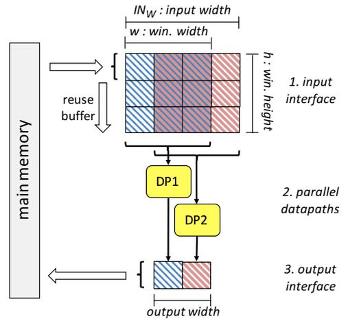
**Figure 4: The automatically generated accelerators include multiple datapaths, executing the loop body of two-dimensional SCoPs.**
