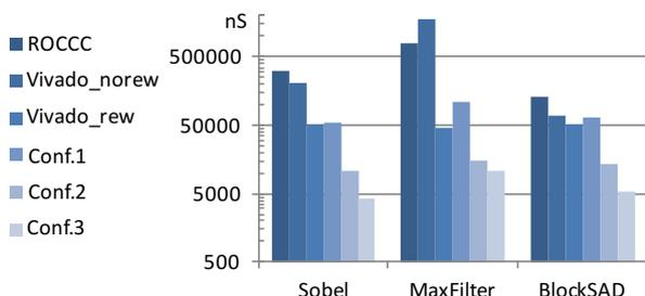
Figure 6: Execution time to process a 100x100 frame.
