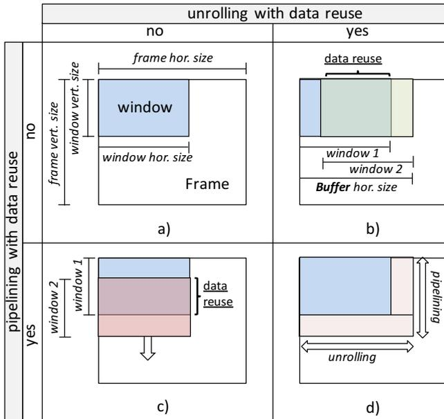
**Figure 3:** At each iteration, sliding window applications process a subset of the input data (a). The managed set of subsequent iterations present a high degree of overlap, both in the horizontal (b) and vertical (c) dimensions. Our framework automatically leverages both, maximising data reuse (d).
